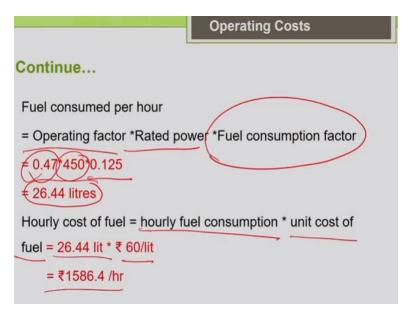
Now let us find what is the fuel consume per hour? So the operating factor multiplied by rated power into fuel consumption factor. So this fuel consumption factor which is determined for the standard conditions may be we are going to adjust it according to your project operating factor and the rated power of the machine. So the fuel consumption factor is nothing but 0.25, it is per horsepower per hour your horse power of the machine is 450 and the operating factor is 0.47.
