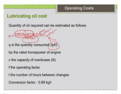
That is the only difference so here you can see the consumption rate is 0.0027 kg per horse power. Accordingly, you have to adjust according to your conditions into horse power into the operating factor into the plus crankcase capacity divided by the number of hours between the changes. And the conversion factor here is 0.89 kg per liter so the final quantity you will get it in liters per hour using this formula.
