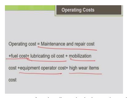
So what are all the components so far we have discussed under the operating cost let us summarize. So maintenance and repair cost your fuel cost, lubricating oil cost all these are consumables, the mobilization cost, equipment operator cost and cost of special items of high wear items. So all these things we have operating cost of the machine.
